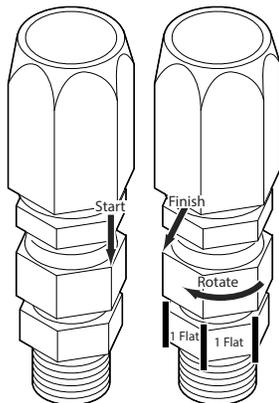
**Caution:** Do not introduce a twist to the hose when tightening the BP261 to the BP208 (or BP242).
