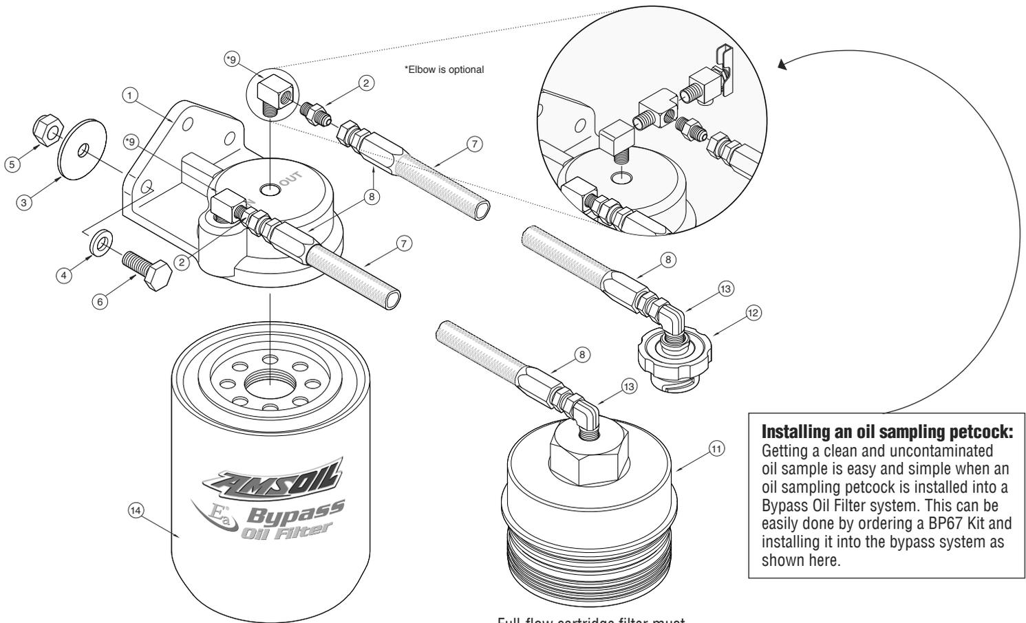
**Installing an oil sampling petcock:** Getting a clean and uncontaminated oil sample is easy and simple when an oil sampling petcock is installed into a Bypass Oil Filter system. This can be easily done by ordering a BP67 Kit and installing it into the bypass system as shown here.
